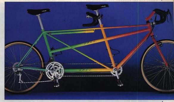
and Nicol penciled in a pair of custom 30-mm oversize seatposts, which resist flex. This allows the Ibis to be sized for extra standover clearance, an essential ingredient for confident off-road riding.
